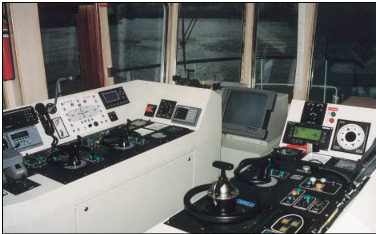
Figure 6 Layout of the bridge, with Master pilot control and independent thruster control handles
